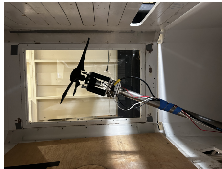
Fig. 10 Experimental setup within the wind tunnel test section.
