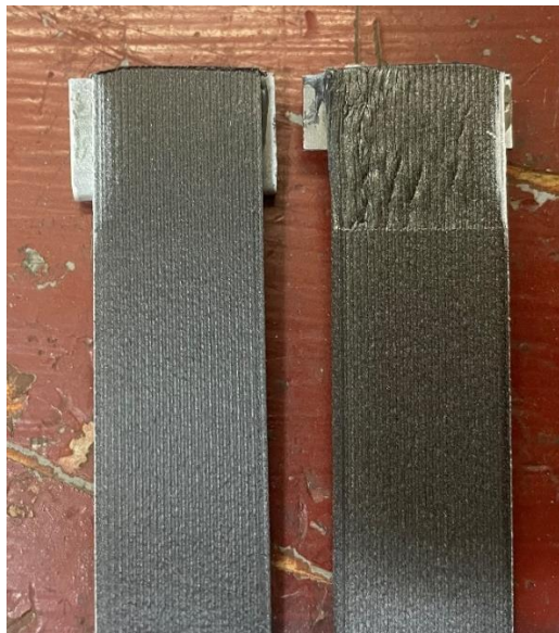
Figure 6. Layer adhesion to polytetrafluoroethylene tape
