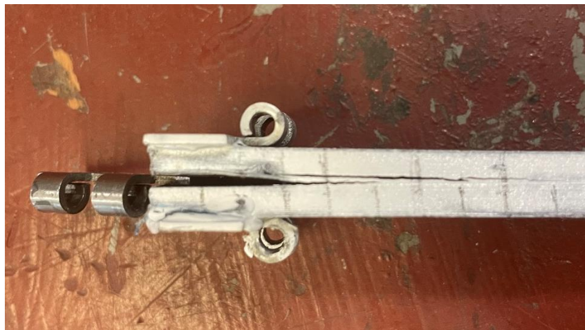
Figure 4. Paint affecting crack propagation
