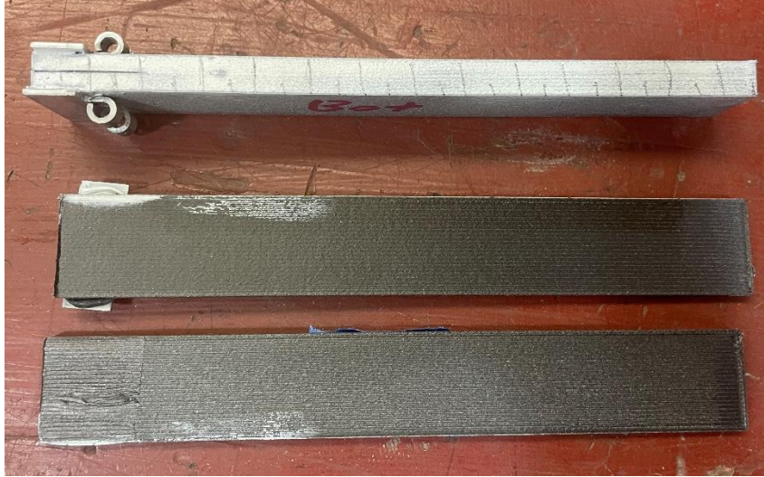
Figure 5. Paint between print layers
