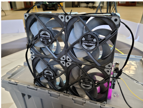
Fig. 4 Computer Fan Module Used for Wind Generation Positioned in Flying Environment
