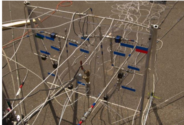
Figure 1. The complexity of an old test stand panel proved to be very tedious to set up and looked very haphazard.
