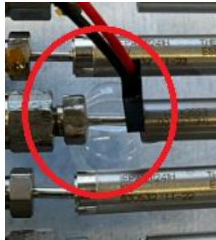
Fig. 4 VISORS Valve Manifold Bubbling During Manifold Assembly Process
