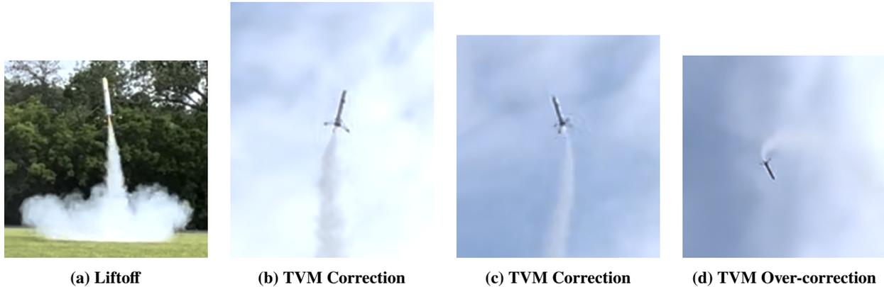
**Fig. 7** TMV reacting to the deviation detected by the IMU sensor onboard, last picture shows an over-correction of TVM
