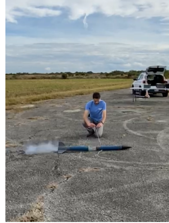
(b) Ejection charge test of the bottom section.
