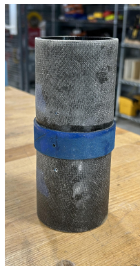
(b) Side view of the tube coupler.
