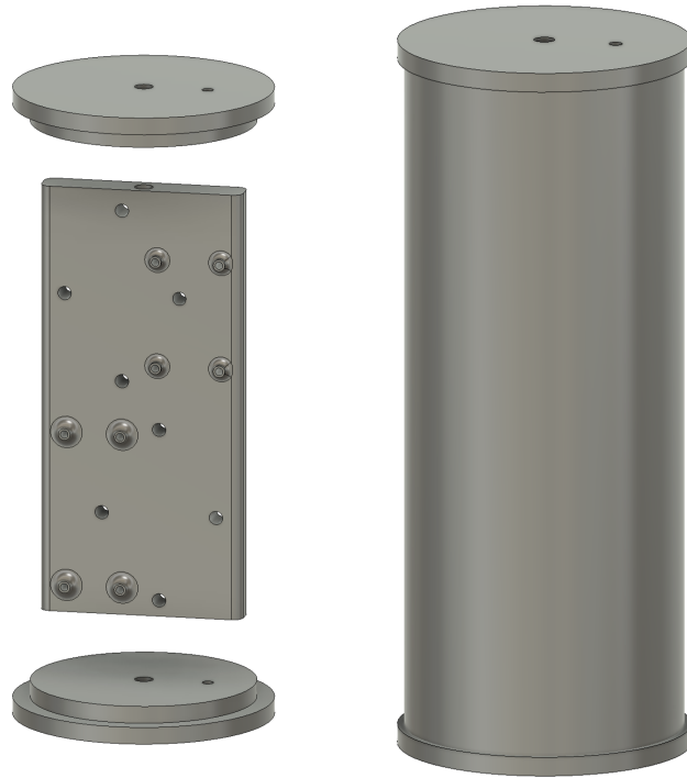
(a) The avionics sled and bulk-heads that sealed the ends of the avionics bay.
