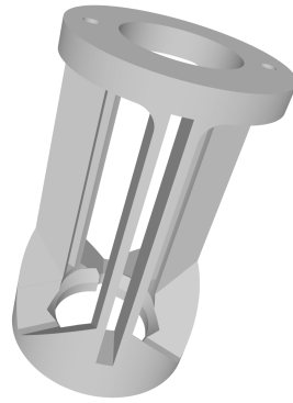
Fig. 4 An image of the 3D printable motor tube holder and fin aligner. A previous member of the Florida Tech AIAA rocket team designed this piece.
